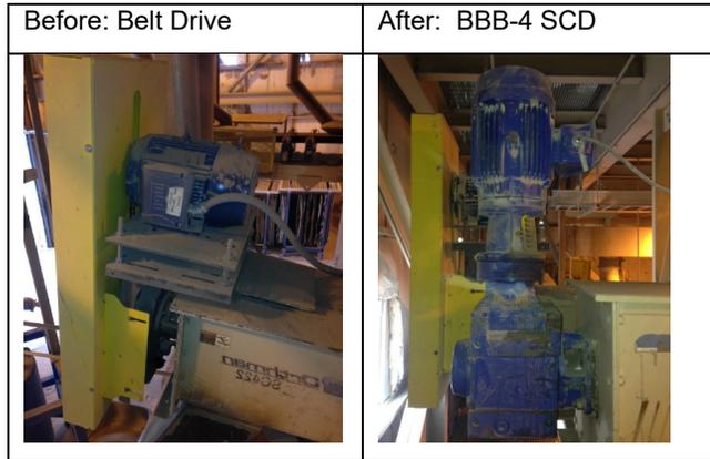
Replacing your belt driven Screw Conveyor Drive (SCD) with a direct driven Sumitomo BBB-4 SCD is a mechanically efficient solution that can reduce opportunities for injuries.
